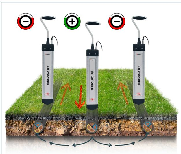
If there are several lines (cables, pipes) located next to each other, it is often difficult to determine which the correct one is. Sometimes the signal from the generator can flow through both lines, but the signal in the lines may be flowing in different directions. With the SignalSelect function, the generator applies a signal that contains directional information. When the device is positioned over the correct cable, a "+" symbol is displayed to facilitate precise identification.
